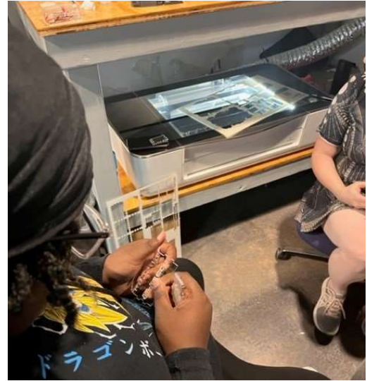
Goodie is assembling a laser cut enclosure after witnessing it being engraved with her name and cut on our laser cutter.
